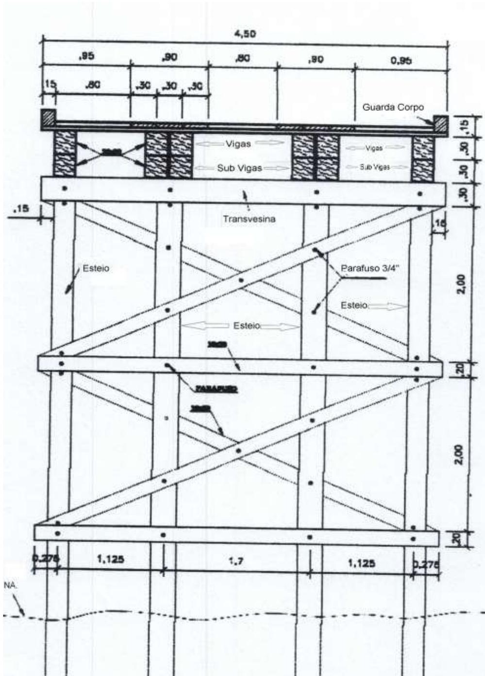
Figura 01: Cavalete c/ 4 esteios - alt. 8,50m a 9,50m
